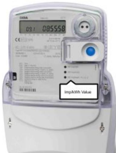
**Imp/kWh Value:** a value describing the number of LED pulses displayed by an energy meter for every kWh of energy that passes through the system, e.g. **1000 Imp/kWh**. Number of pulses are detected and recorded by a meter reader, and energy usage over a given period can be calculated.
